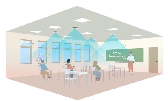
Figure 3: Illustrative example of a UVGI luminaire application
