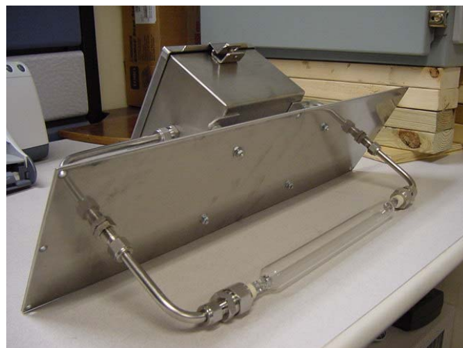
Figure 2: UV lamp installation.
