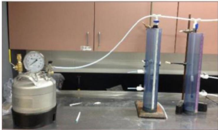
Dissolved Air Floatation Reactor
